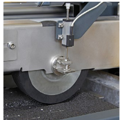
Detail of the motorized lifting system that raises the wheel assembly at the end of the test, making the use of hoists obsolete.
