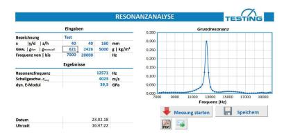
By mechanical stimulation of resonance frequencies, the RA100 Concrete measures according to the Impact Resonance Method easily and quickly the sound velocity. Compressive strength, static and dynamic modulus of elasticity are determinated directly and with calibration values.
