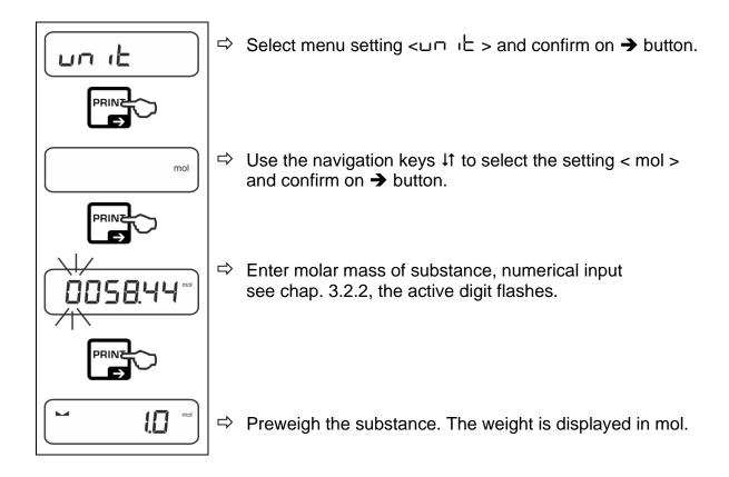
The required settings can also be defined quickly and conveniently by pressing the key (without calling up the < up it> menu), see chap. 10.3.2.
