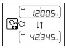
⇒ Using **S** button, it is possible to switch over between the enabled unit 1 and unit 2.
