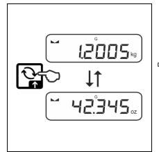
⇒ Using ≤ button, it is possible to switch over between the enabled unit 1 and unit 2.
