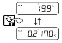
The required settings can also be defined quickly and conveniently by pressing the so button (without calling up the < un it > menu), see chap. 10.3.2.
