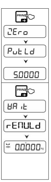
⇒ Acknowledge selection by → button.< ☐E ¬□ >, <P \ L \ □ > followed by the weight value of the adjustment weight to be placed will be displayed.
