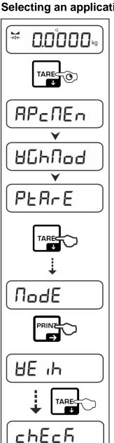
⇒ Press the **TARE** key and hold it until  $< AP \subseteq \Pi \in \Pi >$  is displayed.
