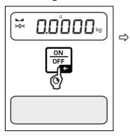
Keep ON/OFF button pressed until the display disappears
