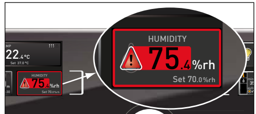
Fig. 21 Humidity monitoring triggered
