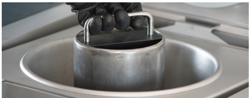
Placing the centrifuge cup into the centrifuge unit
