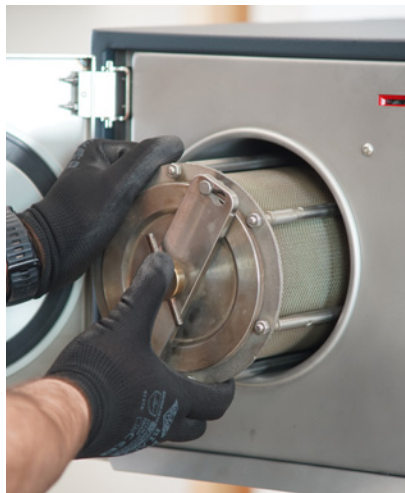
Placing the washing drum into the machine
