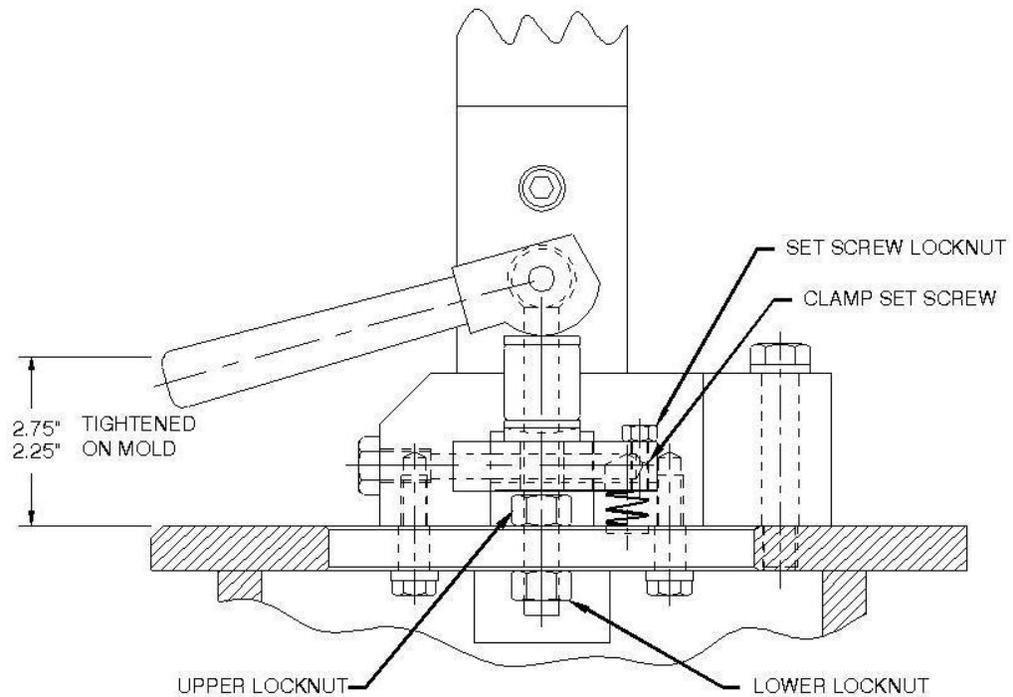
**Figure 7.4a: Mold Clamp Components**
