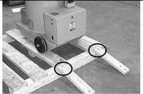
Step 3: lock the handles to the frame of the compactor with the safety pins in the handle.
