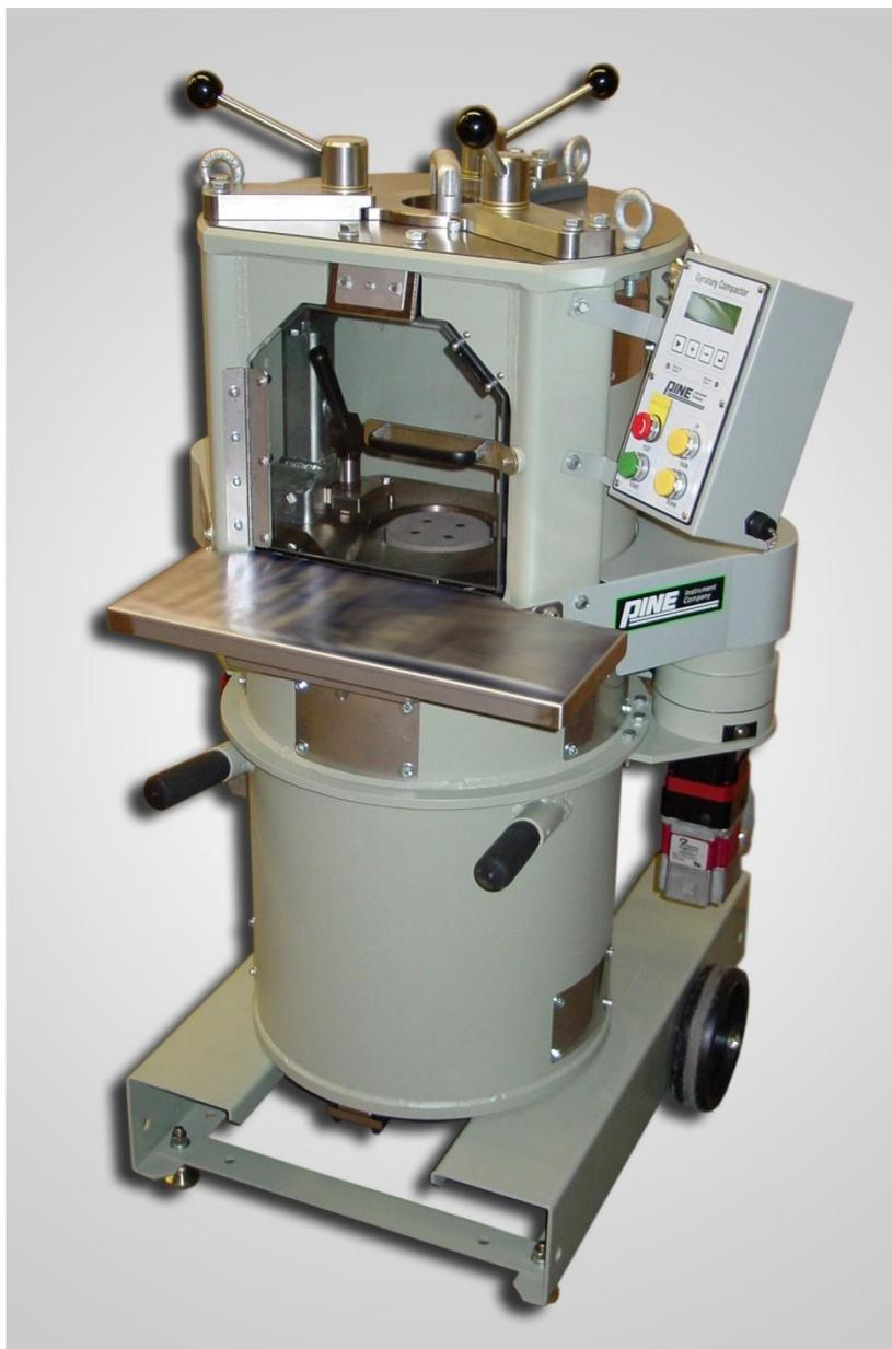
Figure 1.1: The Pine AFG2 SUPERPAVE™ Gyratory Compactor
