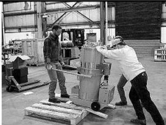
Step 6: Remove the safety pins and side the handles into the frame mounts.
