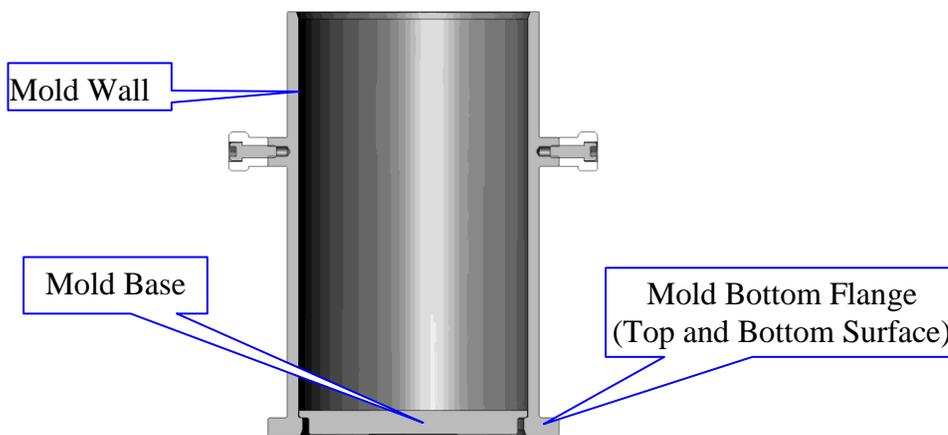
Figure 7.2: Cleaning Diagram-Mold
