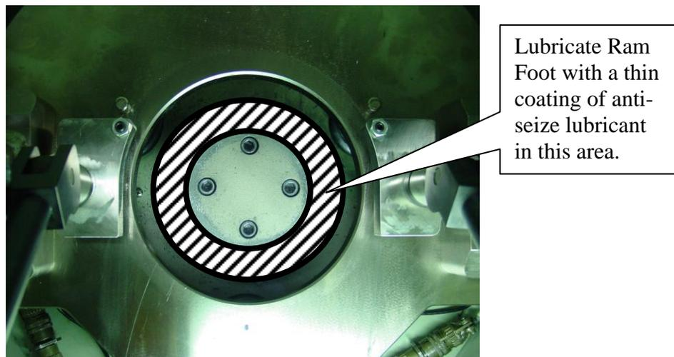
Figure 7.3: Ram Foot Lubrication
