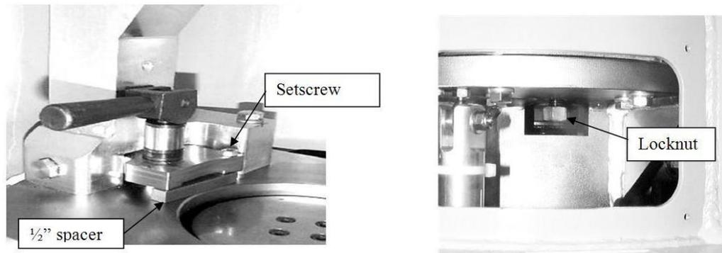
**Figure 7.4b: Mold Clamp Adjustment**
