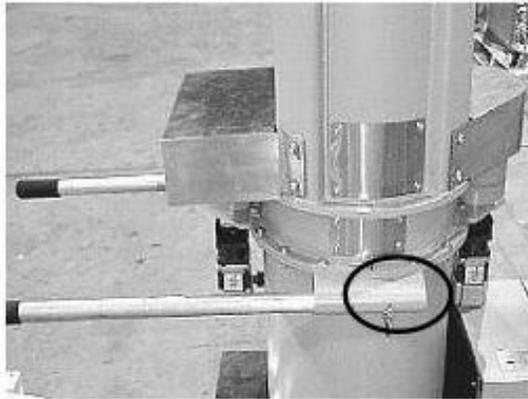
Step 4: Slowly roll the compactor to the edge of the pallet. Use spotters to help balance the load.
