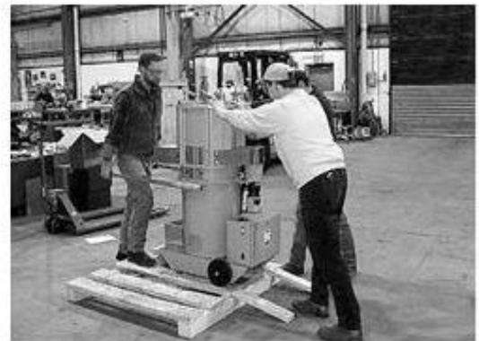
Step 5: Roll the compactor down the ramps very slowly using spotters to control the compactor.
