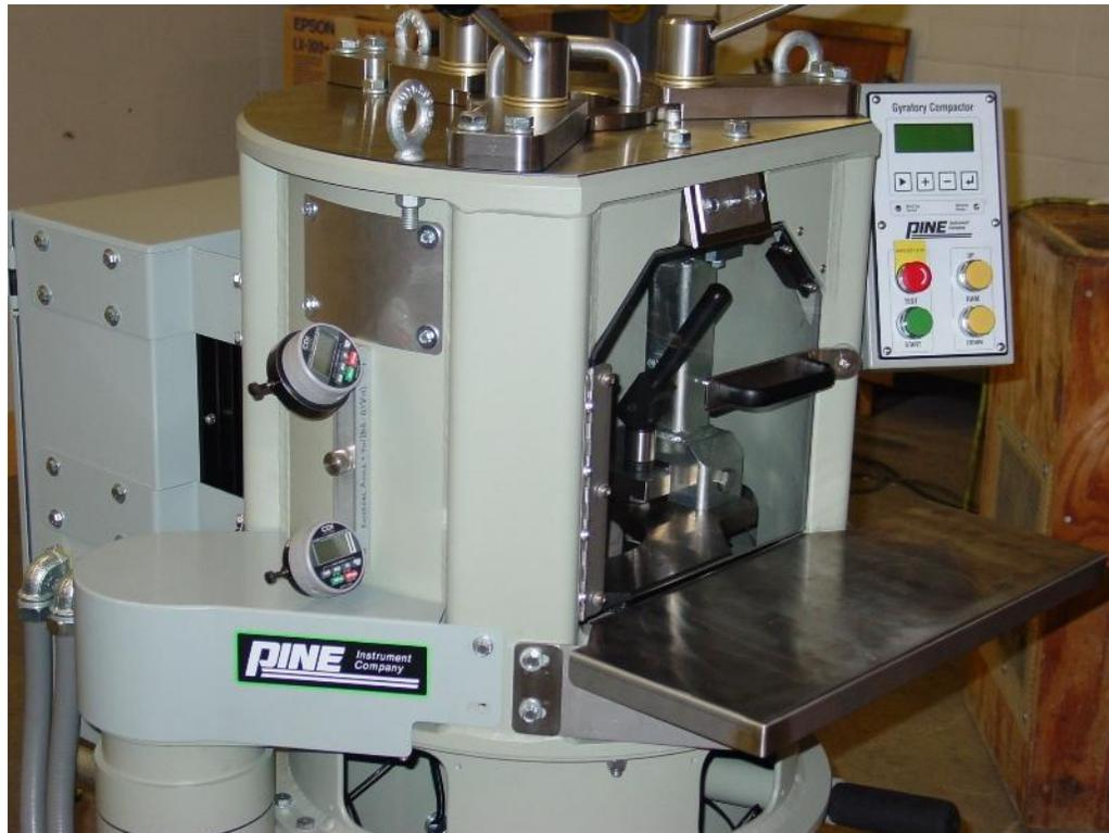
Figure 6.4: External Angle Verification
