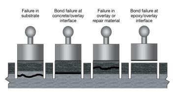
For example "B 100%" indicates a complete failure in the overlay or repair material.
