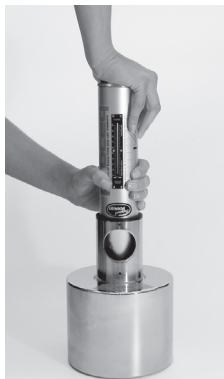
Fig. 3.1 Performance check of the concrete test hammer (model N/L shown)
