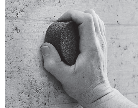
Fig. 2.1 Preparing the test surface
