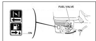
Turn the fuel valve to the ON position.
