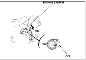
Put the engine switch on ON, and make sure the emergency switch on the board of the machine is in the correct position.
