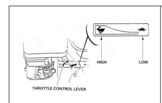
Move the throttle control lever slightly to the left.
