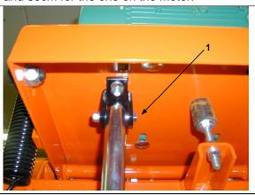
Then tighten the adjustment bar on the back of the head (1) with the M8 screw supplied for this purpose.
