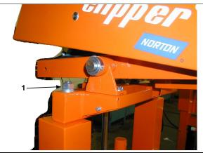
Place the head on the two posts of the frame, so that the threaded rods pass through the holes designed for this purpose in the head. Tighten the M20 (1) nuts to fix the head.
