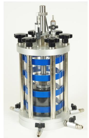
*CRS - Constant Rate of Strain cell (26-WF0360/AD) fitted in triaxial cell 28-WF4070 with sumersible load cell, displacement transducer and mounting bracket*
