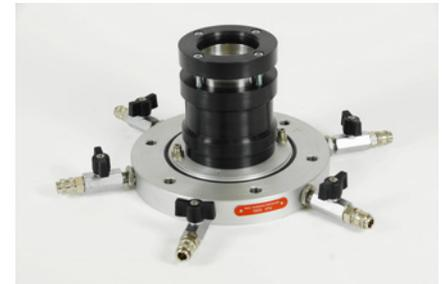
*CRS - Constant Rate of Strain cell (26-WF0360/AD) fitted on base platen of triaxial cell 28-WF4070*
