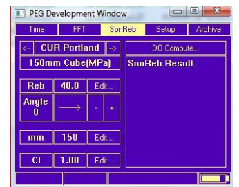
SonReb menu to evaluate the concrete strength combining the ultrasonic and concrete hammer measurements
