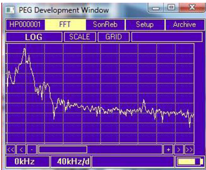
FFT menu for displaying Fast Fourier Transform of the signal
