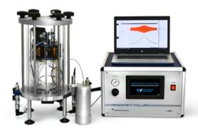
**RESUNANT CULUMN** Combined resonant column and torsional shear device
