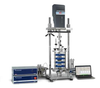
Automatic dynamic triaxial testing machine
