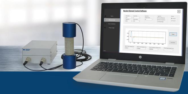
Bender elements allow you to measure the maximum shear modulus ( $G_{max}$ ) of a soil sample in order to evaluate its stiffness.  $G_{max}$  — typically with shear strain levels of about 0.001% — is a key parameter in low-strain dynamic analysis used to predict soil behaviour or soil structure interaction during earthquakes, explosion or machine and traffic vibrations.
