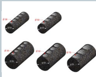
Taking transversal coring samples using the suitable accessory
