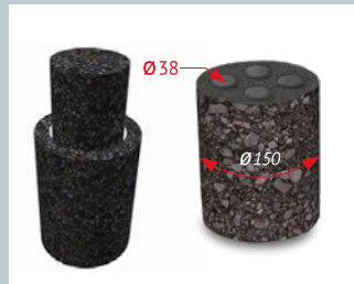
Coring cylindrical asphalt samples using the suitable accessory
