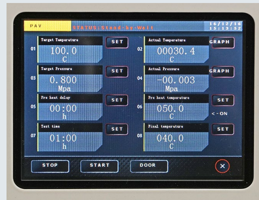
Temperature and pressure target values vs actual values.
