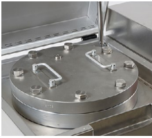
Detail of certified pressure vessel and cover locking switch
