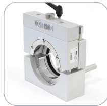
Interlayer bonding / Shear bond Test (Leutner)
