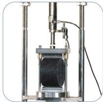
Indirect tensile strength/ IDEAL-CT
