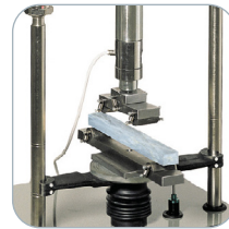
Flexural test on soil - cement specimens
