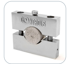
Splitting tensile test of intact core specimens
