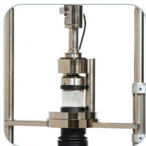
Compression on low strength mortar mixes
