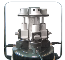
Elastic Modulus on mortar and Cement
