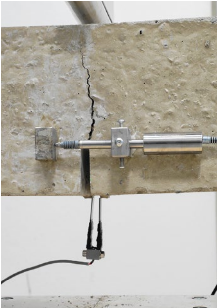
Detail of CMOD testing to EN 14651
