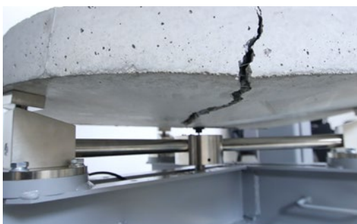
Detail of round slab test to ASTM C1550 travel displacement transducer
