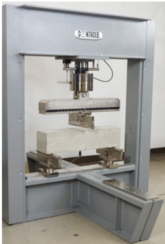
Testing FRC beams to EN 14651
