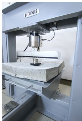
Energy absorption test to EN 14488-5
