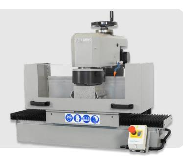
The New Controls Grinding Machine 'bench' single phase model provides laboratories with a compact and safe alternative to bulkier models traditionally available on the market.
