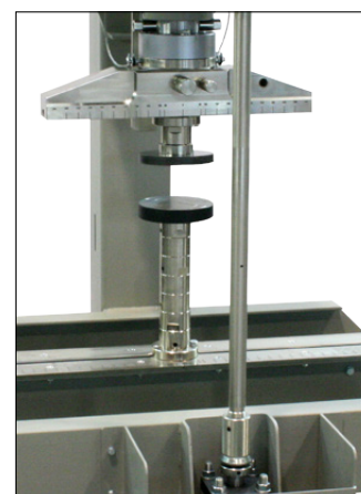
300 kN UNIFLEX frame (50-C1601/FR) fitted with accessory for compression tests (50-C1601/4 and 50-C1601/KIT)
