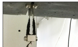
CMOD test, detail of clip gauge transducer (82-P0331/E)
