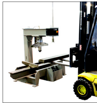
Easy specimen loading with forklift
