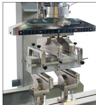
1300 kN UNIFLEX frame (50-C1601/FR) fitted with accessories for kerbs testing 50-C1601/2, 50-C1601/KIT and 50-C1601/3)
