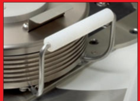
**Especially user-friendly:** The grinding sets of 100 ml volume and larger for the FRITSCH PULVERISETTE 9 are equipped with handles.
