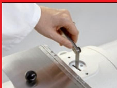
**Especially convenient:** Easy gap width check from the outside (e.g. with thickness gauge)
