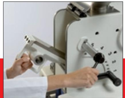
Saves time and energy: **The especially simple crushing jaw removal** takes only seconds and requires only two hand motions to ensure particularly simple cleaning – fast and thorough.
