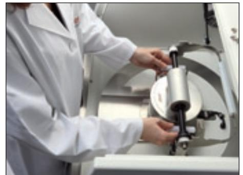
**Especially ergonomic:** The grinding sets of the FRITSCH PULVERISETTE 9 with significantly reduced weight are placed on a carriage and slide into the defined final position. The operating position is adapted to body height – which is back-friendly and saves energy and time.
