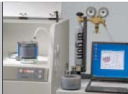
The PULVERISETTE 4 grinding in inert gas
