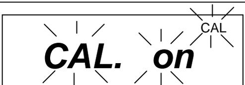
The display changes automatically from [**CAL.on**] to [**CAL.oFF**]
