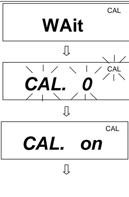
Rotate the turn knob on the right side of the balance in to position **CAL**.
