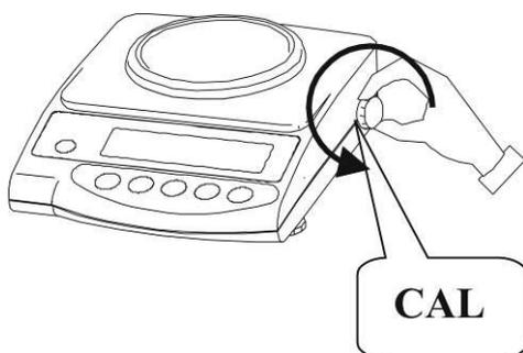
Adjustment is carried out automatically. [**CAL.on**] will appear flashing.
