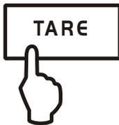
⇒ Unload the balance and press the **TARE** button, the zero display appears.
