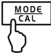
Using this function the weight of a tare vessel is stored. Even after turning off/on the weighing balance will continue working with the saved tare value.
