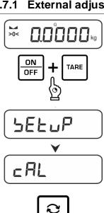
⇒ Press and hold the TARE and ON/OFF buttons simultaneously to enter the setup menu.
