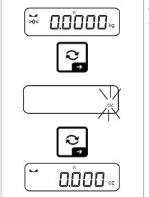
The unit for quick selection can be determined when the  $\rightleftharpoons$ -button is shortly pressed for the first time.
