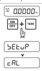
⇒ Press and hold the TARE and ON/OFF buttons simultaneously to enter the setup menu.
