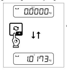
⇒ Keep the ≥ button pressed until the display shows the gross weight value.
