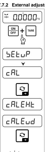
⇒ Press and hold the TARE and ON/OFF buttons simultaneously to enter the setup menu.
