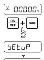
⇒ Press and hold the TARE and ON/OFF buttons simultaneously to enter the setup menu.
