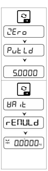
⇒ Acknowledge selection by → button. < ☐E □ ⊃, < P □ E L □ > followed by the weight value of the adjustment weight to be placed will be displayed.
