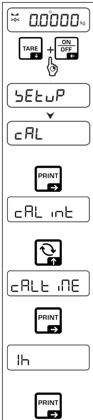
⇒ Press and hold the TARE and ON/OFF buttons simultaneously to enter the setup menu.
