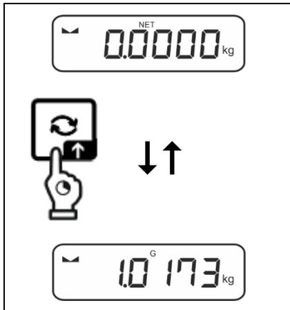
⇒ - Press and hold the ↻-button until the display shows the gross weight value.
