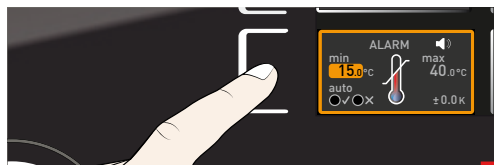
Fig. 17 Reset button for the mechanical temperature limiter (TB)
