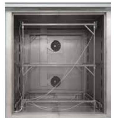
Pluggable frame for measurement for air circulation chamber furnace N 7920/45 HAS
