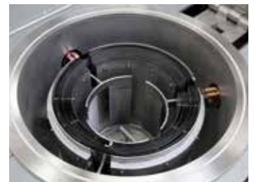
Cylindrical retort with tungsten heating
