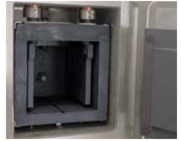
Graphite heating chamber
