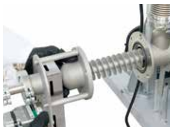
Screw-conveyor with adjustable speed
