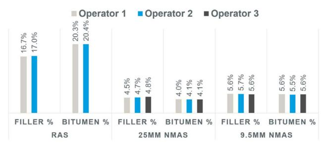
Figure 3 The Impact of Operator Error on Asphalt Binder Content and Percentage of Fines
