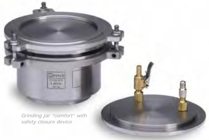
Grinding jar "comfort" with safety closure device
