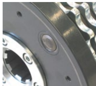
Drum with replacement bushes = longer service life
