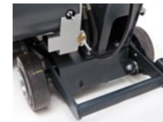
Foot lever for transport position = fast machine relocation
